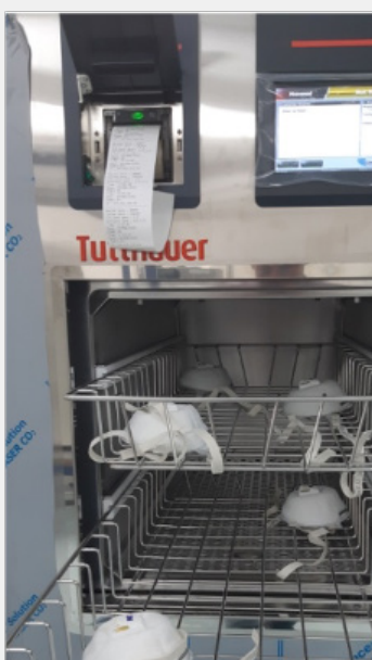
Pic. 1: N95 FFR masks positioning in Tuttnauer's 160L PlazMax sterilization chamber
