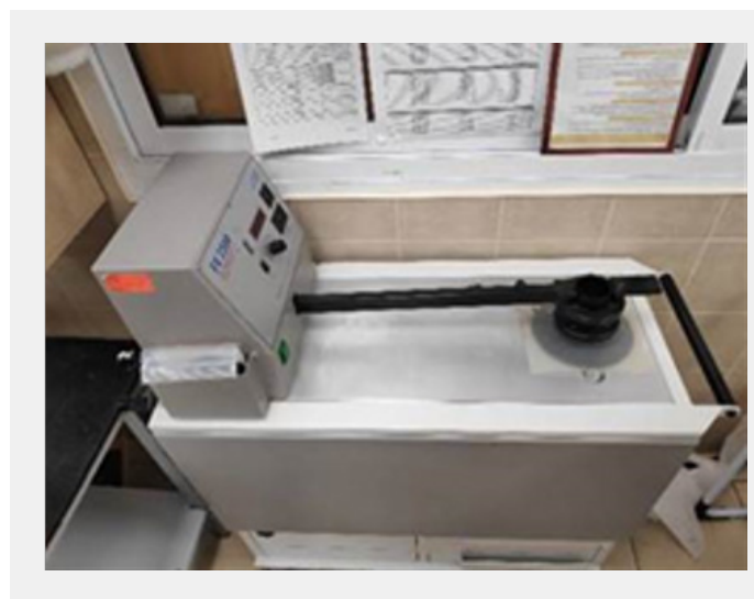
Pic. 2: FX 3300 Air Permeability Tester III, by TEXTEST Instruments
