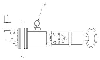
It is important to clean the hole of the air trap, as described at point 2 before starting operation of the autoclave, for the first time.
