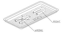
20. Packs should be placed upright on the tray. They should not be touching each other or the Chamber walls. There should be about 1" between packs for proper steam circulation.
