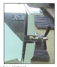
9. At the end of the cycle a buzzer rings for approximately 5 seconds, the START light switches OFF. The air outlet valve is opened to prevent formation of a vacuum.
