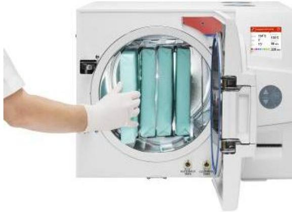
23. Small packs can be placed directly on the tray in an upright position. They should not be touching each other or the Chamber walls. There should be about ½” to 1” between packs for proper steam circulation.
