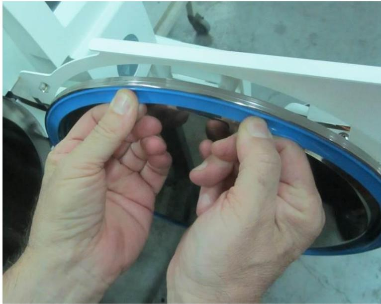
2. Clean the groove of any remnants of the old gasket (use a plastic scraper and plain water as needed).
