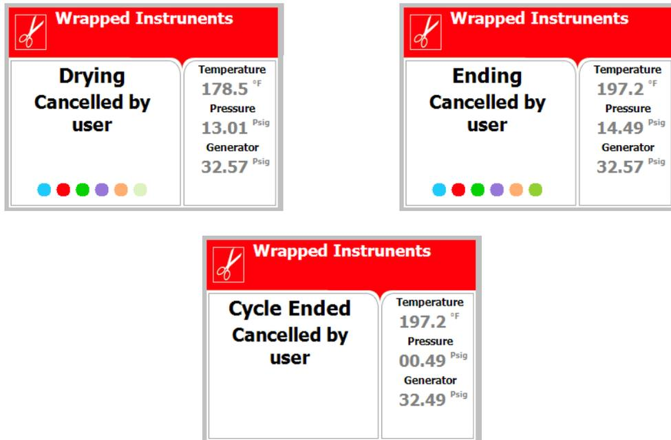
**Note:** The user will have to press the **START/STOP** key, after the mandatory 1-minute drying, to clear the message and unlock the door.
