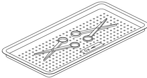
10. Make sure that all instruments remain apart during the sterilization cycle. Surfaces that are hidden because items are covering other items will not be exposed to the steam and will not be sterilized.
