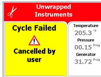
**Note:** The user will have to press the **START/STOP** key, after the mandatory 1-minute drying, to clear the message and unlock the door.
