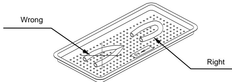
21. Cassettes or packs should be placed on the tray rack in place of the trays. They should not be touching each other or the Chamber walls. There should be about  $\frac{1}{2}$ " (1.25cm) between cassettes or packs for proper steam circulation.
