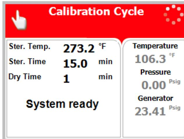
This program is only for use by a technician with the proper test equipment to aid in calibrating the autoclave. This is a shortened cycle with a long sterilization phase at 273.2°F (134°C) and no drying. (1-minute drying is still required to remove residual steam from the chamber).
