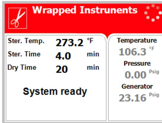
For wrapped instruments, pouches, and materials, when the instrument manufacturer recommends autoclaving at temperatures of 273.2°F (134°C) with a drying stage.
