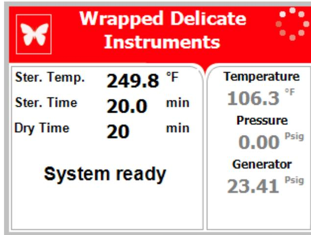
For wrapped Handpieces when the instrument manufacturer recommends autoclaving at temperatures of 249.8°F (121°C) with a drying stage.
