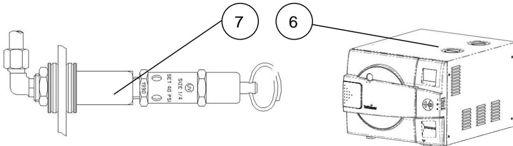
In case more water is accidentally filled above the blue area or safety valve, decrease the water level by draining the reservoir before starting a cycle (see sec. 10.4).
