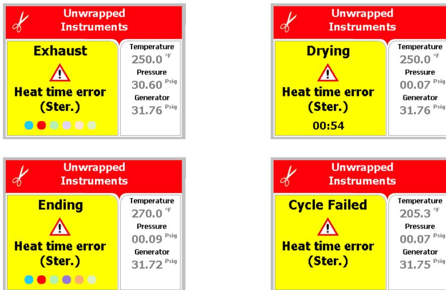
**Note:** The user will have to press the **START/STOP** key, after the mandatory 1-minute drying, to clear the message and unlock the door.
