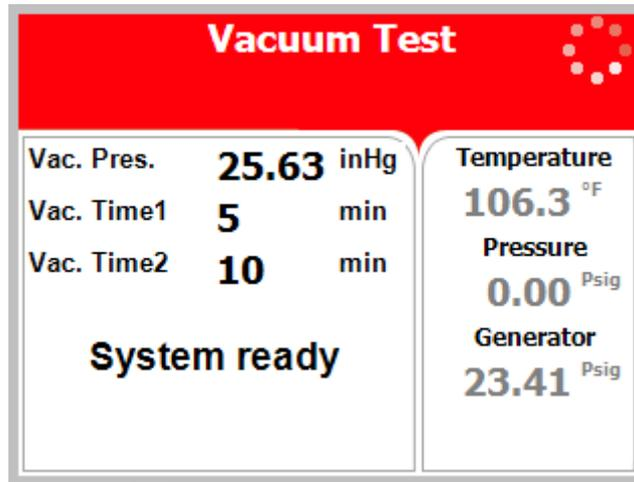
Vacuum is produced in the chamber, down to P1=2.47psi (0.17bar). At this stage all the valves close. The autoclave remains in this stage for 5 minutes. This period enables the condition in the chamber to reach equilibrium. After the 5 minutes have elapsed, the printer records the pressure that is referred to as P2. At this point the test begins and lasts 10 minutes. At the end of the test, the printer records the results. The pressure at the end of the test is referred to as P3.
