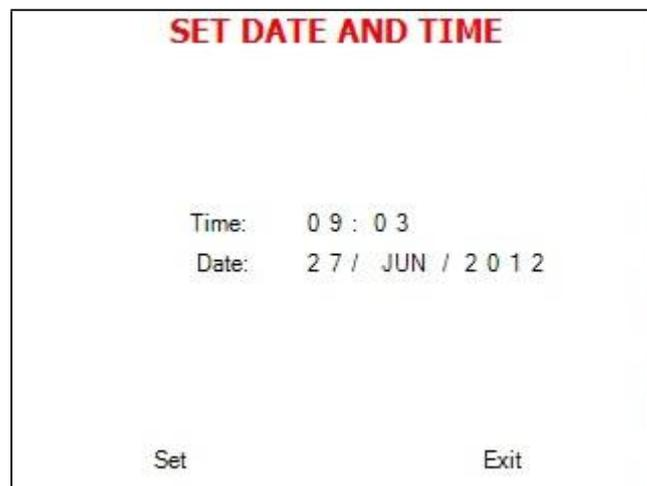
The time is displayed in the upper row in the form “HH:MM”. The time is in a 24 hour format (i.e. 14:30 = 2:30 PM)
