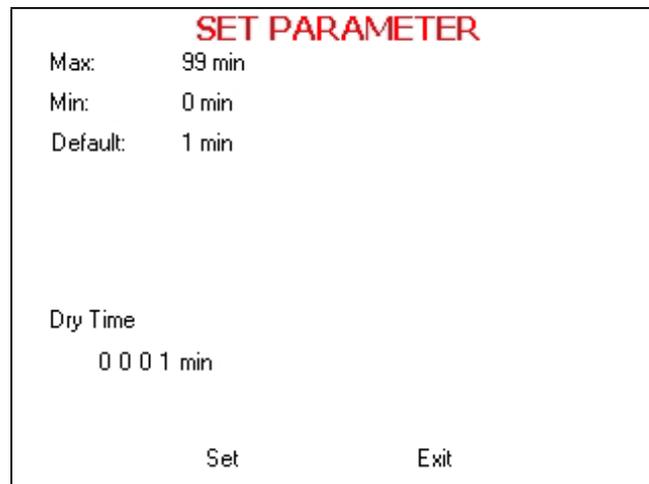
The Set Parameter screen shows the name of the parameter to be changed; it shows the maximum, minimum, and default values for this parameter. It also shows the current parameter setting.
