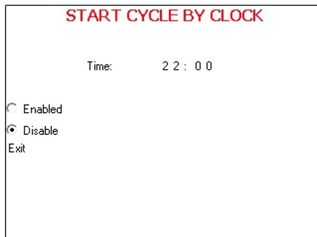
The time is displayed in the form "HH:MM". The time is in a 24-hour format (i.e., 14:30 = 2:30 PM).
