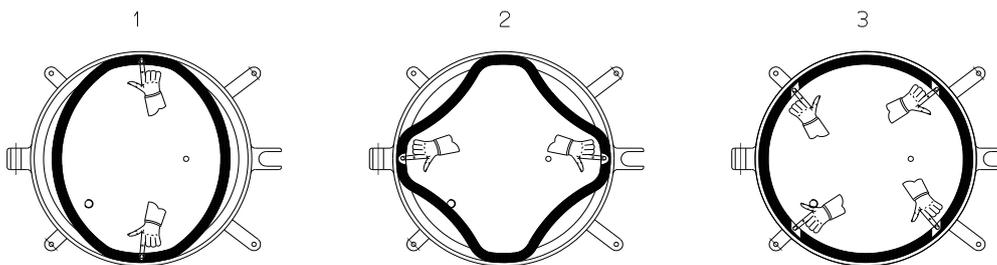
Place the gasket inside the groove and press it in with a finger following the pattern above.
