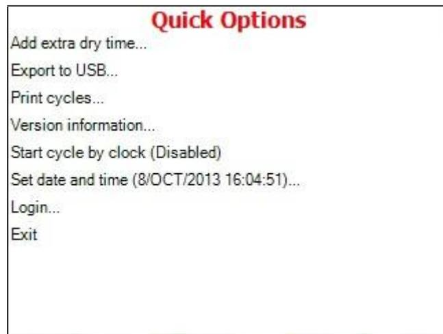
2. To exit this screen or any screen in this section, press the UP or DOWN key to move the cursor to Exit and press START/STOP key.
