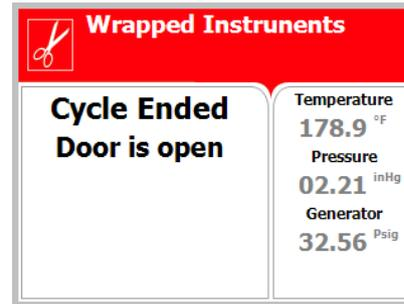
**Note:** The user will have to press the **START/STOP** key, after the mandatory 1-minute drying, to clear the message and unlock the door.
