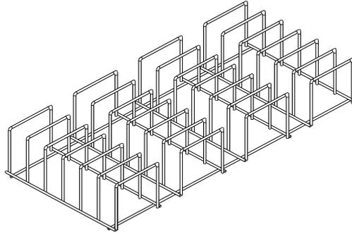
18. Empty canisters should be placed upside-down, to prevent the accumulation of water (see the figure below).
