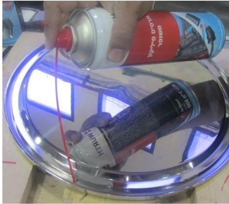
**Note:** It is necessary to use a silicone based lubricant such as Würth Silicone Lubricant or Dow Corning 111, when installing the door gasket.
