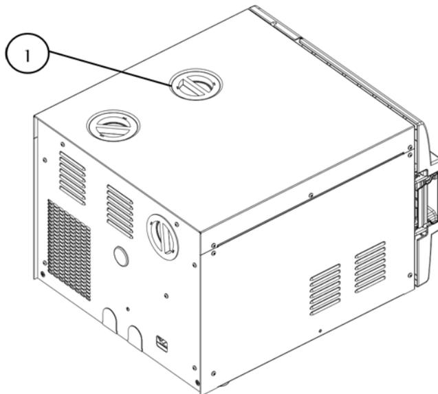
To prevent the safety valve from becoming blocked, it is necessary to open the valve under pressure. This will allow the steam to escape clearing the seat of the valve. Once per month, perform the following procedure:
