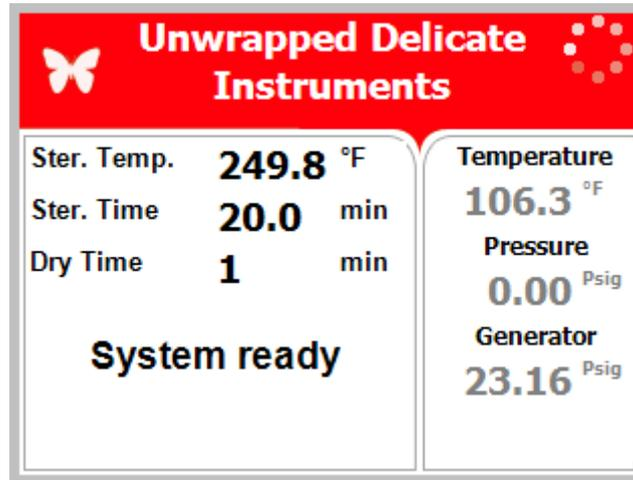
For unwrapped delicate instruments, when the instrument manufacturer recommends autoclaving at temperatures of 249.8°F (121°C) and no drying stage is required (1-minute drying is still required to remove residual steam from the chamber).
