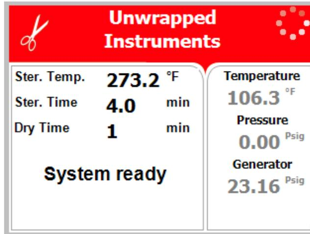
For unwrapped instruments and materials, when the instrument manufacturer recommends autoclaving at temperatures of 273.2°F (134°C) and no drying stage is required (1-minute drying is still required to remove residual steam from the chamber).
