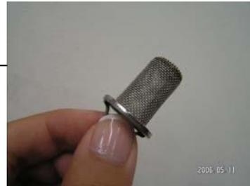
The strainer element is located on the back of the chamber
