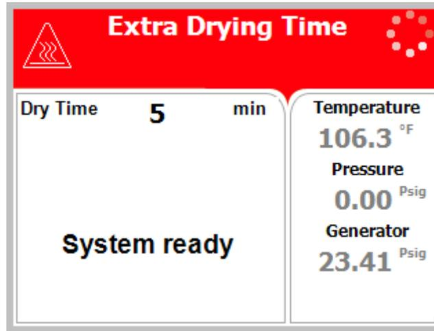
For all loads when the load requires additional drying after the cycle is completed.
