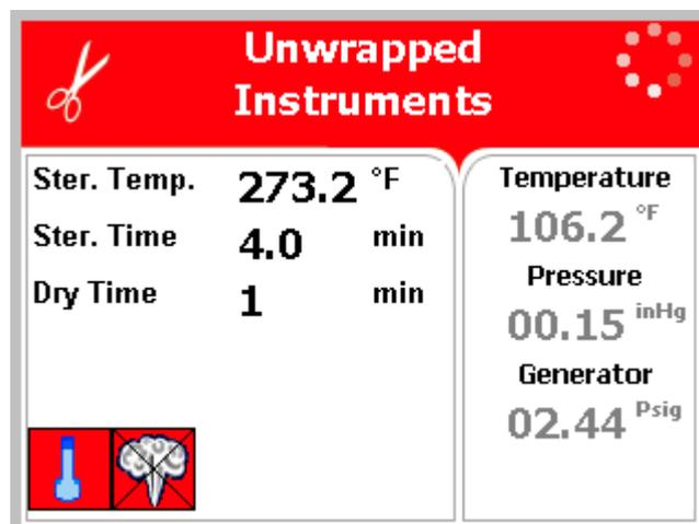
When the unit is turned on the pre-heating begins. The steam generator begins heating and the symbol
