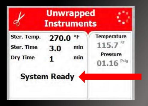
This machine is equipped with an electronic door lock. The door will not open when the power is off or the display screen does not read System Ready
