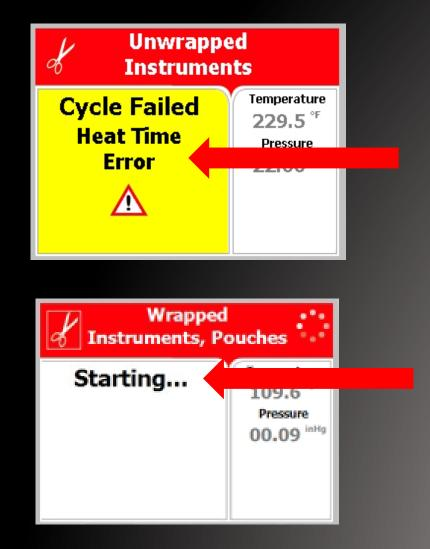
**Problem:** This message is displayed if the chamber cannot reach the required temperature within the preset time.
