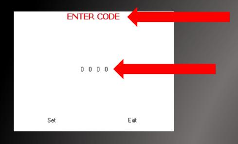
Step 2 Enter Code screen is now displayed 0000 is displayed on the screen with the cursor blinking on the right digit
